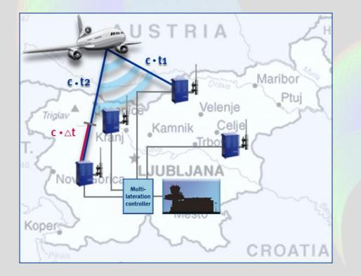
Time delays are used for estimation of the position of a plane.
